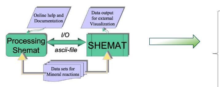
General structure of the simulation package SHEMAT / Processing SHEMAT (Clauser 2003)
