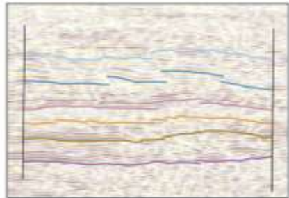
Interpretation Workflow 1: Horizon interpretation leaving fault gaps.
