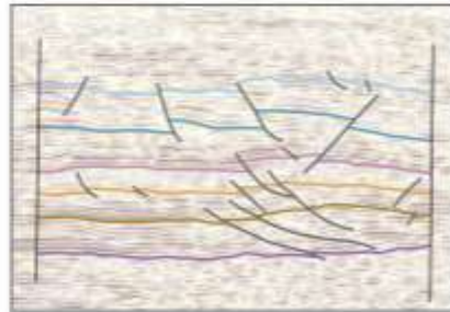
Interpretation Workflow 2: Fault interpretation linking gaps.
